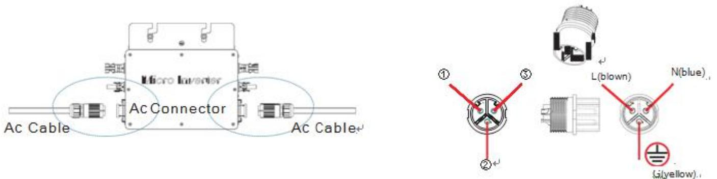
**Step4** Plug the AC output line to main AC cable;
