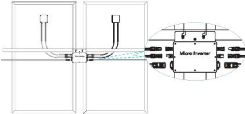
**Step2** Connect the two DC terminal of the PV to the inverter, positive to positive, negative to negative. Show below:
