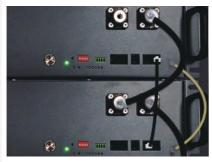
③ Connect the batteries with the battery communication wires.
